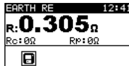
Figure 7.13: Example of earth resistance measurement result
