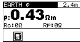
Figure 7.15: Example of specific earth resistance measurement result
